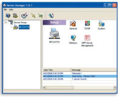
Clicking the "Setup" icon on the tool bar will show the selected Print Server's setup items on the right side of the window.
